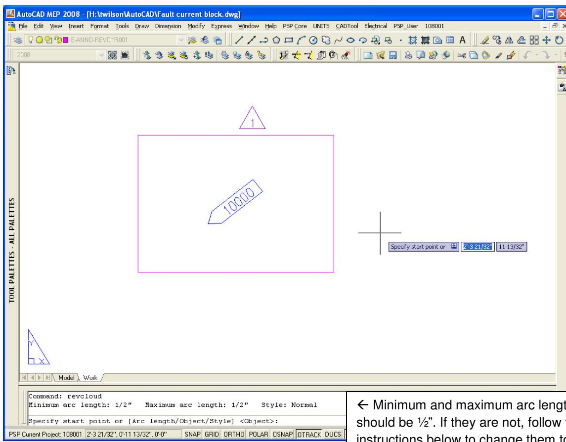
The minimum arc length and maximum arc length should both be  $1/2"$ . If they are not, type **A** to change the arc length:
