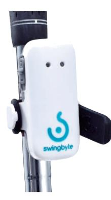
Swingbyte weighs less than an ounce, and attaches to the club shaft just below the grip. Swing the club, and as you make impact with the ball, the sensor transmits a digitized version of your swing via Bluetooth to your phone, which displays clubhead speed, clubface angle, and more. \$149 (includes one year of service); swingbyte.com
