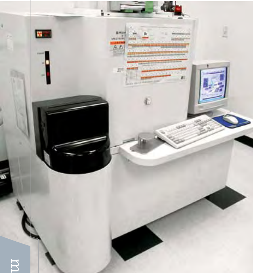
MMR-SRF unit-2. A lab-model x-ray fluorescence spectrometer. Photo courtesy of Massachusetts Materials Research, Inc.
