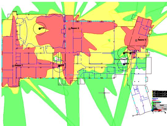
*A tool such as Motorola LAN Planner, part of the Motorola RF Management Suite, simplifies the planning and design of a WLAN.*
